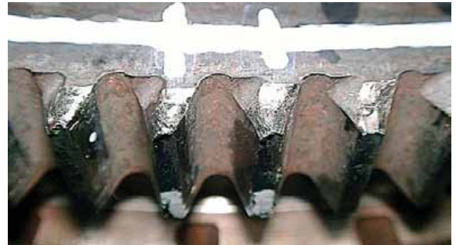
Examples of worn ring gear teeth.
